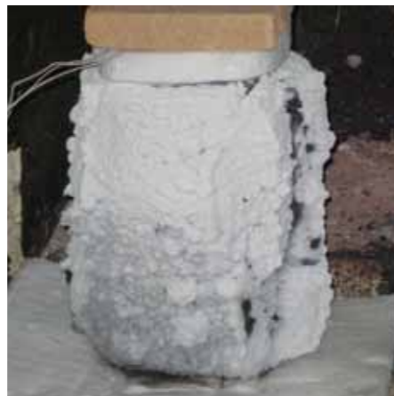
Heated steelwork producing char
